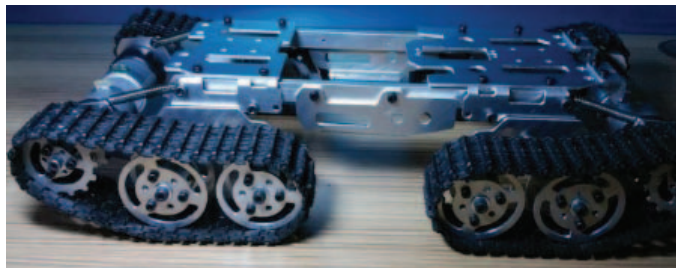
Fig. 4. AMBOA frame without sensor array.
