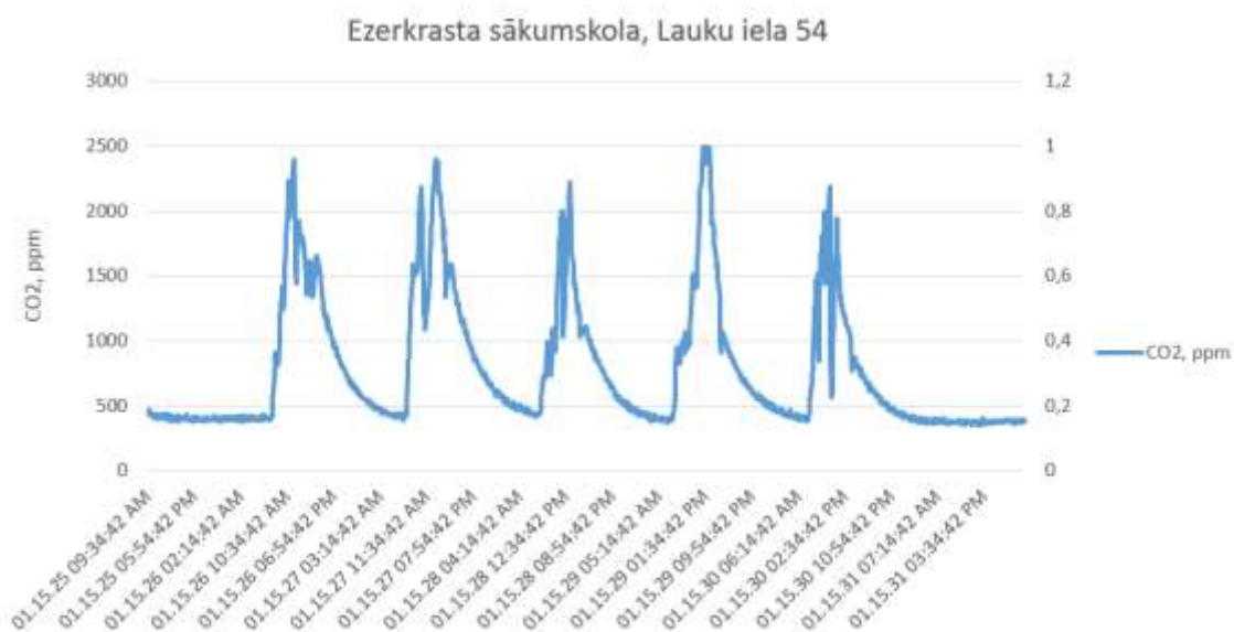
CO 2 measurements in Ezerkrastu primary school building
