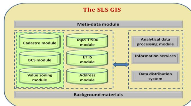
Topo 500 module – Topographic information in scale 1:500 module BCS module – Building cadastral surveying module ET IS module – Encumbered Territories IS module Fig.4: SLS GIS structure. [17]
