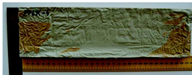
Figure 1. A composite polypropylene-perforated steel material – plane element.
