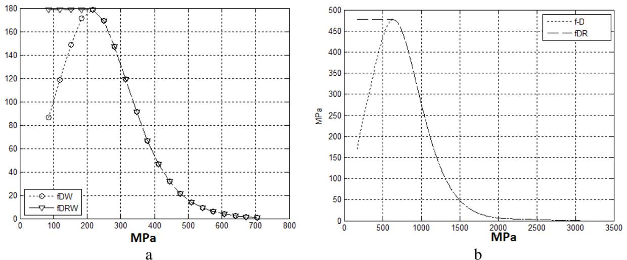
**Fig.4.** The residual (-▼- fDRW) and 'teoretical' (-o- fDW) Daniels' function for damaged LEs (a) and the same (-- fDR) and (... fD) for mixture of undamaged and damaged LEs (b).
