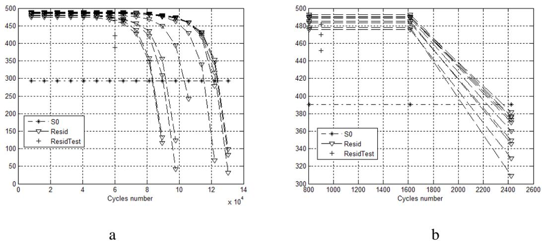
**Fig.3** The nominal cycling stress level (-\*- S0), the 10 examples of random residual Daniels' function (-▼- Resid) and result of test of residual stress (+ ResidTest) as function of cycles number.
