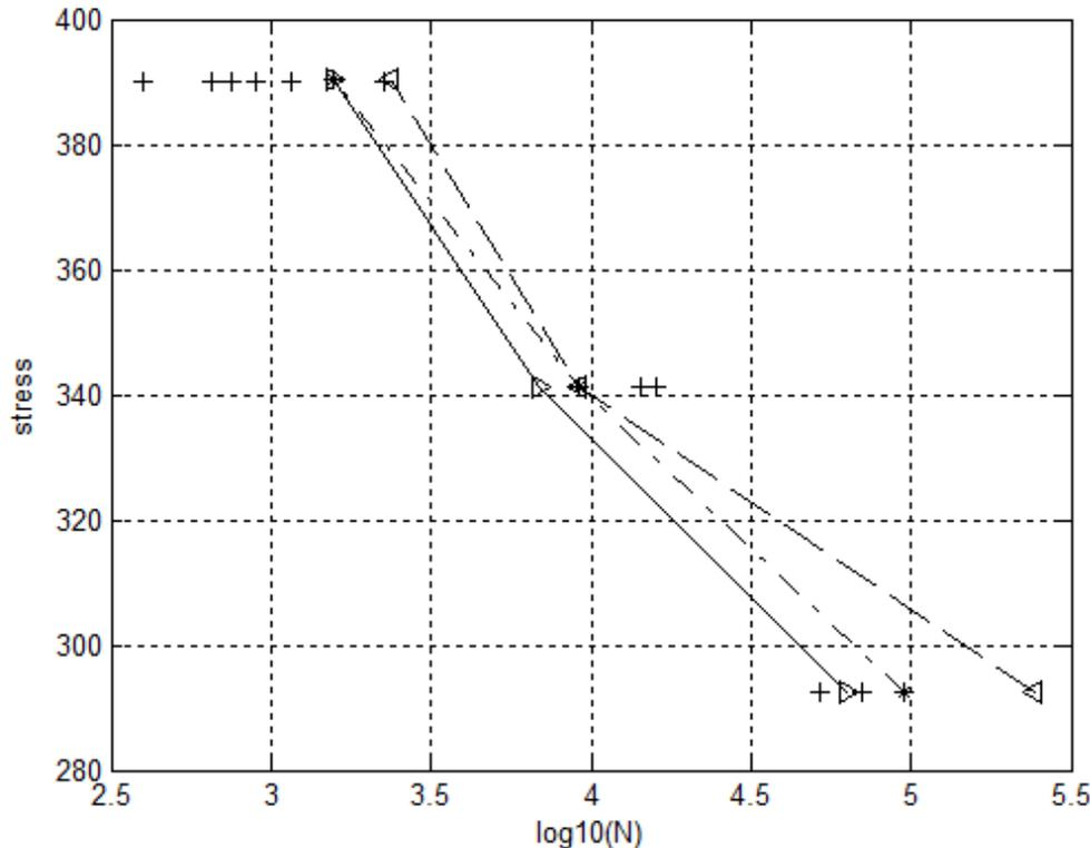
**Fig. 5.** The result of Monte Carlo calculation of fatigue curve (▶ is the smallest value,\* is the mean value,◀ is the largest value) and the result of fatigue test (+) .
