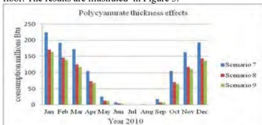
Figure 3. Polyisocyanurate thickness effects on energy consumption
