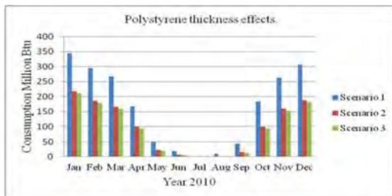
**Figure 1.** Polystyrene thickness effects on energy consumption
