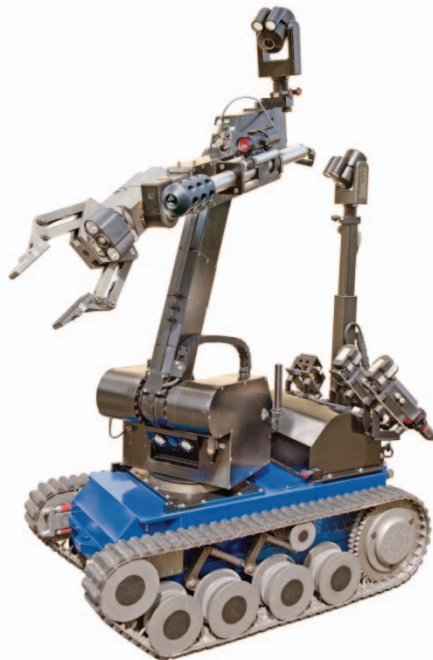
Fig.4. COBHAM's heavy duty EOD robot, similar in autonomy and power requirements to the ISH robots outlined within the paper.
