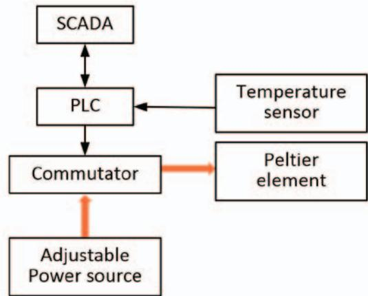
Fig. 5. Temperature Control System.
