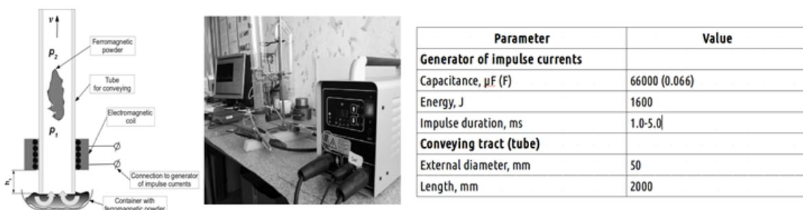
Figure 6: A sequence of operations for powder coating manufacturing by means of electromagnetic pulsed fields.
