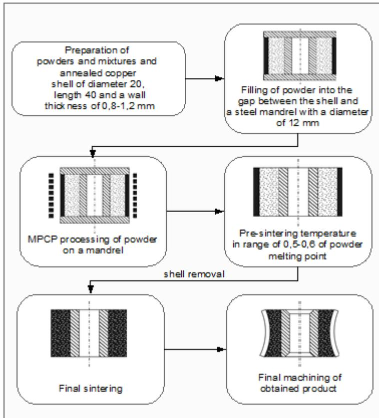
Figure 5: A sequence of operations for powder coating manufacturing by means of pulsed electromagnetic fields.
