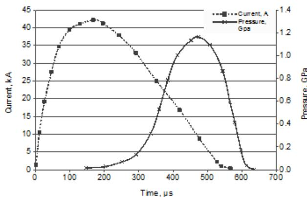
Figure 3: Change of pulse current of  $I$  and electromagnetic pressure  $P$  at flat pressing on the electromagnetic equipment at Riga Technical University.
