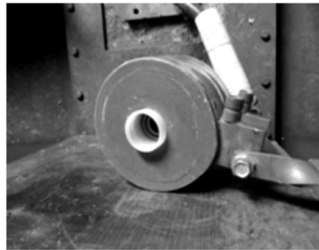
Figure 2: Coil used for radial compaction of powder materials (University of applied sciences of Zwickau, Germany)
