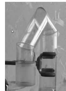
Fig. 6. Cylindrical coil (internal diameter: 50 mm) connected to powder and metallic parts PEMF generator.
