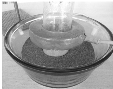
Fig. 6. Cylindrical coil (internal diameter: 50 mm) connected to powder and metallic parts PEMF generator.
