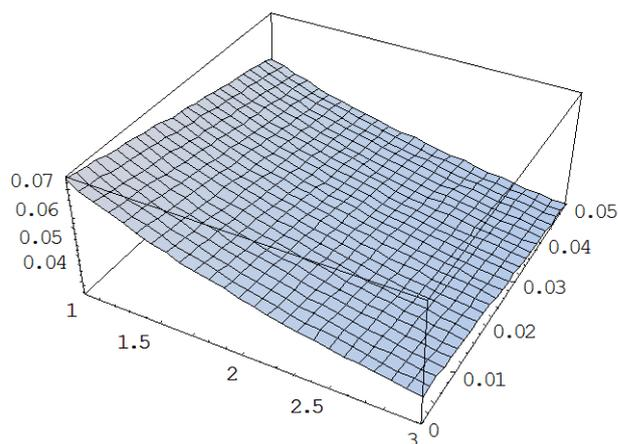
Fig. 10. Marginal stability surface for the case  $1/R = 0.03$  and different values of  $\beta$  and  $B$ .
