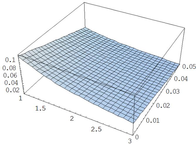
Fig. 5. Marginal stability surface for the case  $1/R = 0.06$  and different values of  $\beta$  and  $B$ .
