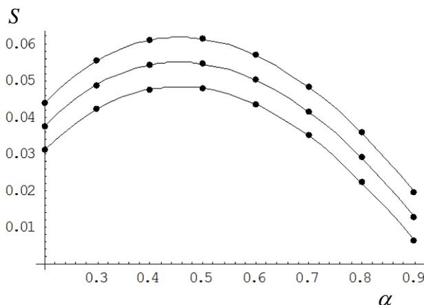
Fig. 6. Marginal stability curves for the case
