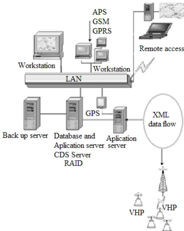
**Fig. 9. Structure of bus control system ASOS**
