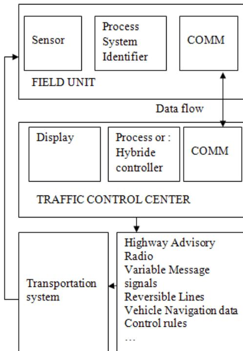
Fig. 2. Functional structure of transport control tool
