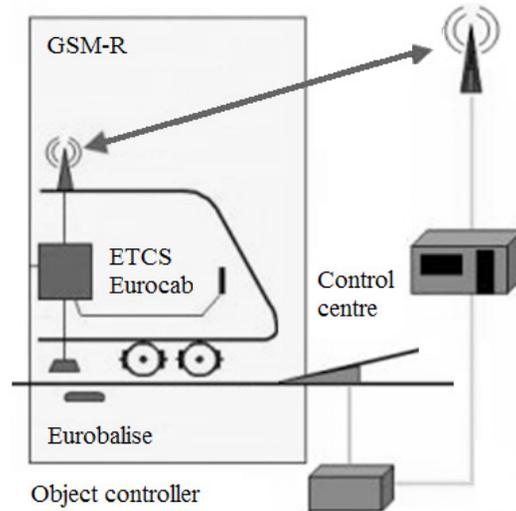
Fig. 6. Signal transmission structure in ETCS
