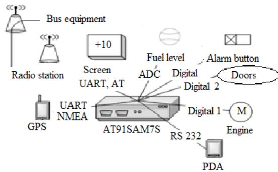
**Fig. 8. On bus equipment with integration in ASOS bus management system**
