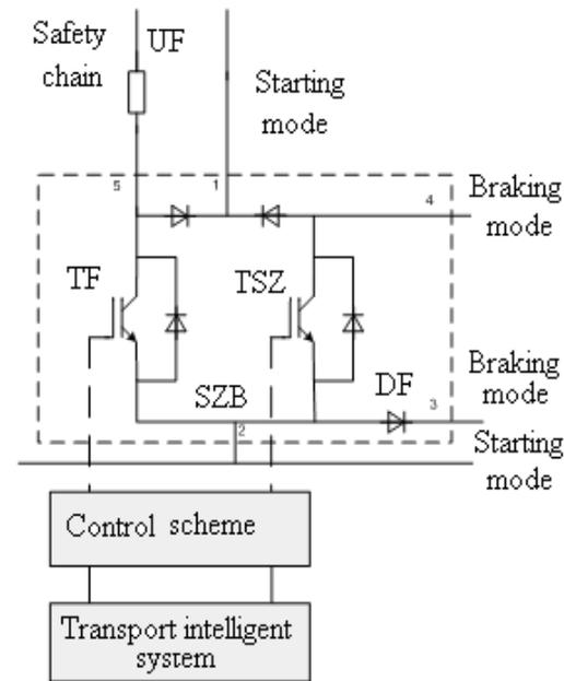
Fig. 7 Functional model of the intelligent transport system equipment for the control of electric energy supply
