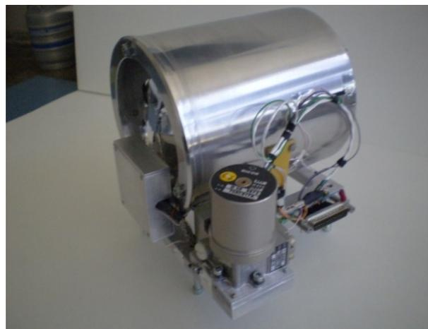
**Fig.3.** Miniature HPGe gamma-spectrometer for space applications
