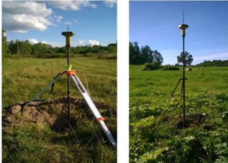
Fig. 5. The practice of static GNSS ellipsoidal height measuring with fixed antenna height
