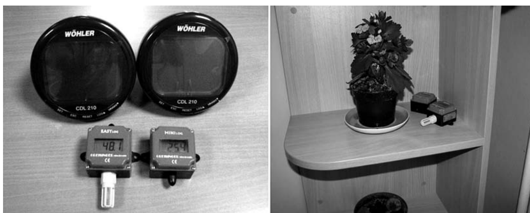
Figure 1. IAQ parameters loggers: Wöhler CDL 210 version 1.1.6, EASYLOG 40RF GSOFT 40K V7.80 and MINILOG GSOFT 40K V7.80
