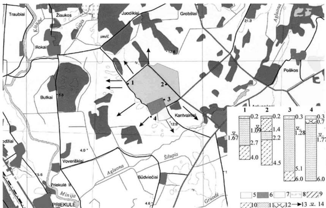
Figure 1. Scheme of the investigation object: 1 - 4 groundwater observation boreholes and their soil profiles; 5 – fields, watered with slurry; 6 – slurry reservoirs; 7 – pig-houses; 8 – plant layer of the soil; 9 – sandy loam; 10 – loam; 11 – sand; 12 – peat; 13 – direction of the groundwater flow; 14 – aquifer level
