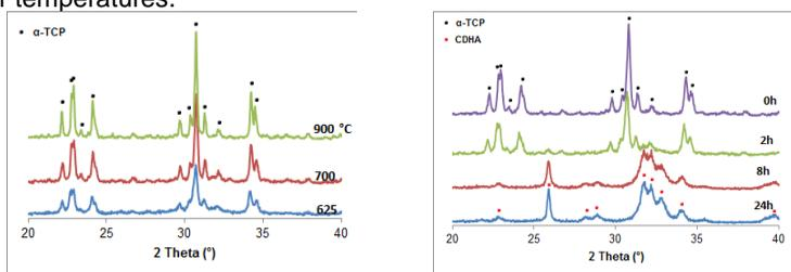
**Fig. 1.** XRD diagrams of  $\alpha$ -TCP powders showing crystallinity increase by increasing the temperature (left); cementation reactions of  $\alpha$ -TCP powder heated at 700 °C (right)
