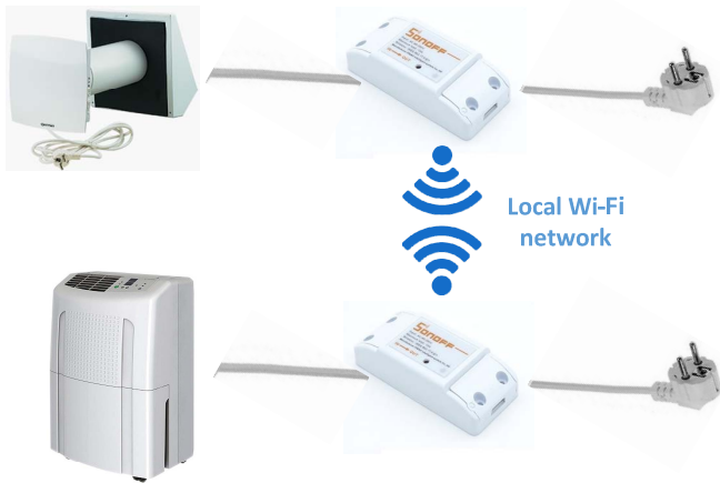
Fig. 7. Sonoff relay connection to ventilation and air conditioner
