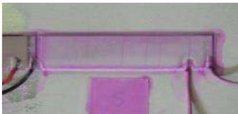
Pic.1. Crack of the PZT after 60000 cycles of fatigue test
