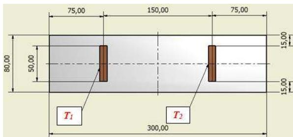
Pic. 2. Test sample of Al2024-T3 1mm sheet
