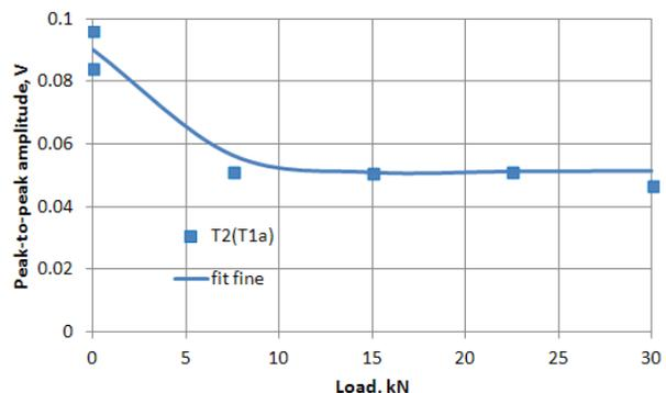
Pic.12. Effect of fatigue crack opening/closing: PPA as a function of load
