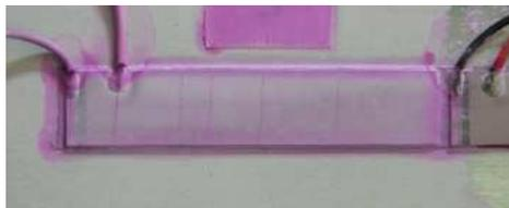
Figure 2. The cracks in piezoceramics after cyclic loading
