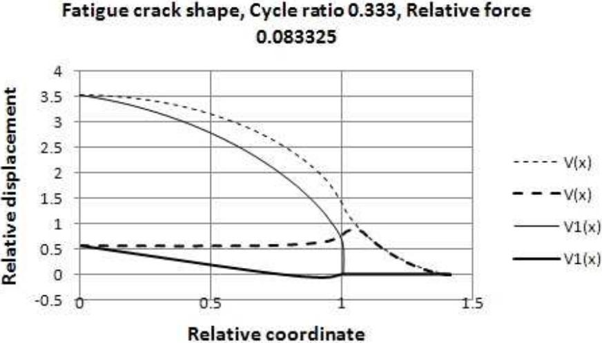
Fig. 16. Fatigue crack shape under maximal load and at further unloading to relative force about 0.083
