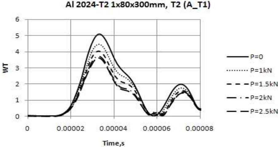
Figure 9. Evolution of WT function during static loading
