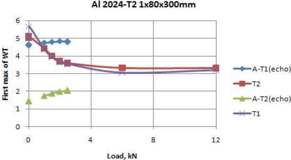
Figure 10. First maximum of WT as a function of load at crack length 27 mm
