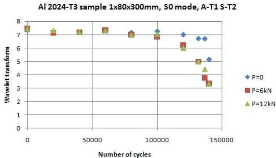
Figure 7. WT first maximum as a function of number of cycles
