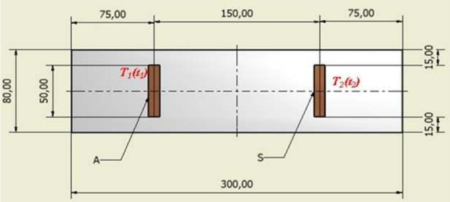
Figure 3. Test sample of Al2024-T3 1mm sheet
