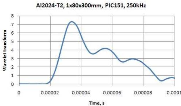
Figure 6. Wavelet transform of transmitted signal
