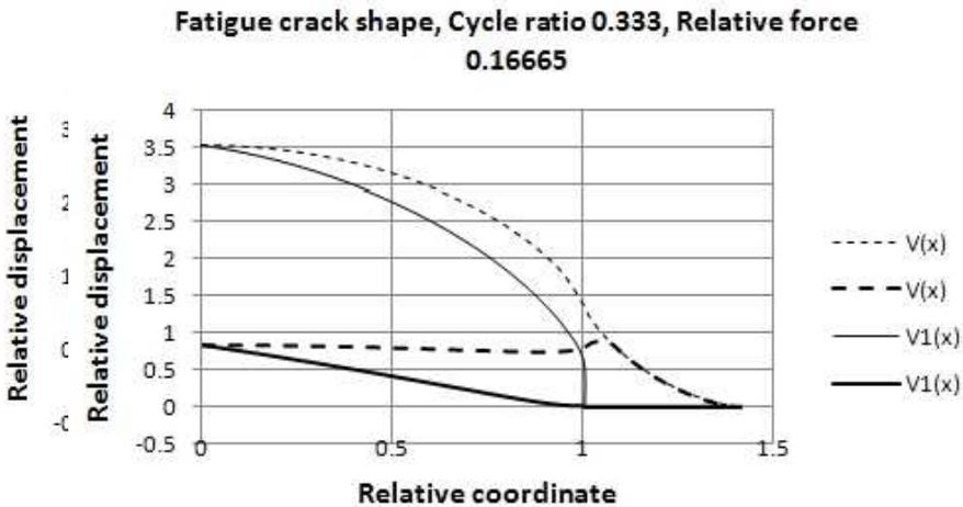
Fig. 13. Fatigue crack shape under maximal and minimal load of cycle
