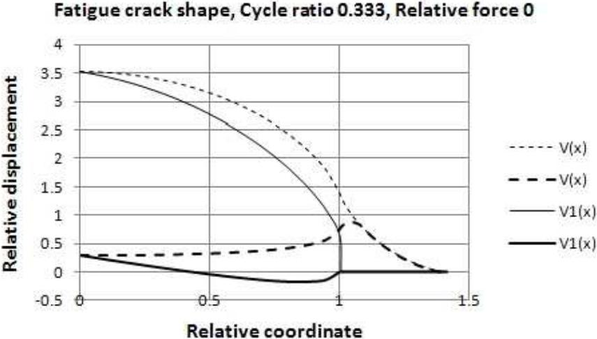
Fig. 17. Fatigue crack shape under maximal load and at full unloading
