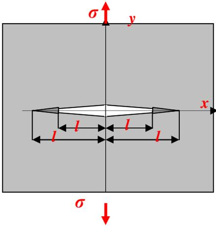
Figure 12. The crack opening and a zone of plastic deformation
