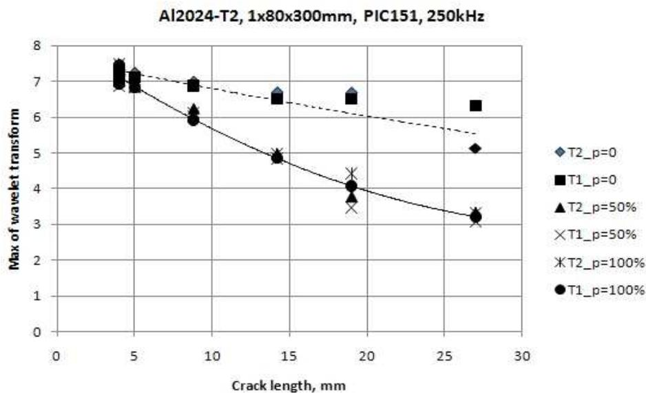
Figure 8. WT first maximum as a function of fatigue crack length
