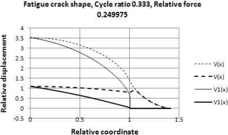
Fig. 14. Fatigue crack shape under maximal load and at further unloading to relative force about 0.25
