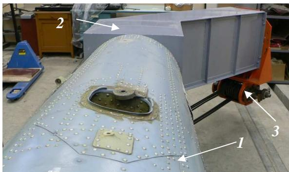
Figure 1. Test set-up of the Mi-8 helicopter tail beam: 1) the tail beam; 2) imitator of the tail propeller beam; 3) mechanical vibrator for exciting of vibration.
