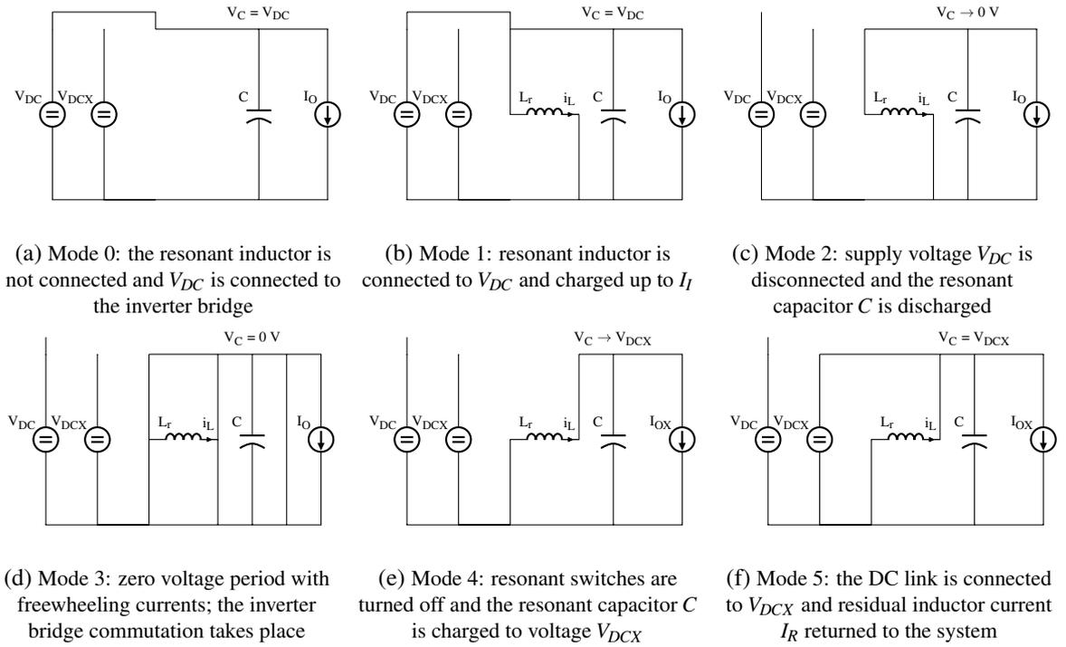
Fig. 7: Operation modes of a DIQRDCLI during a single resonant cycle; here  $V_{DC1} = V_{DC}$  and  $V_{DC2} = V_{DCX}$
