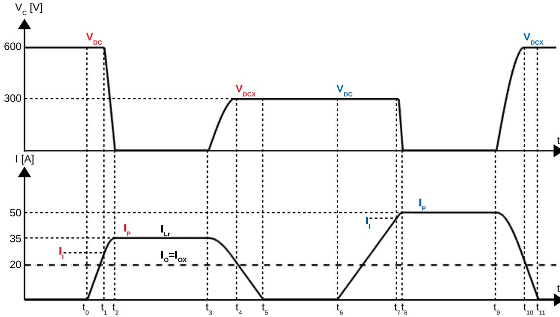
Fig. 6: Simulated waveforms of a single operational cycle
