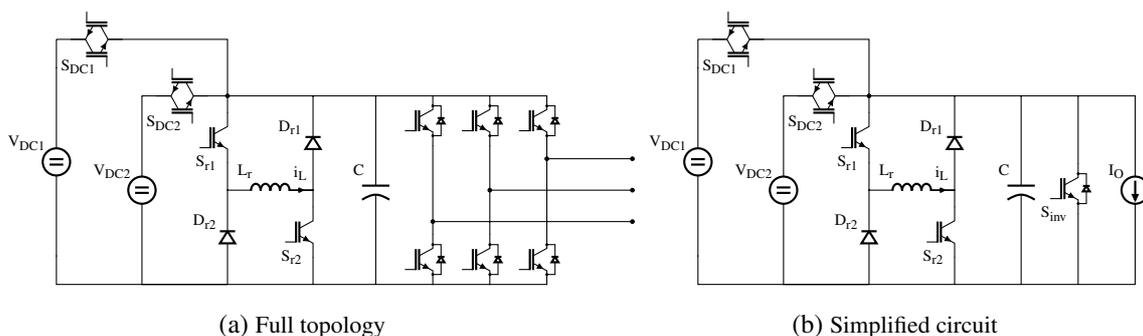
Fig. 5: A DIQRDCLI example topology using the three switch quasi-resonant DC Link from [13]
