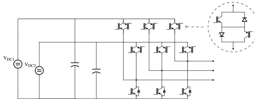
Fig. 2: Circuit topology of a hard switched multiple DC inputs inverter as described in [5]
