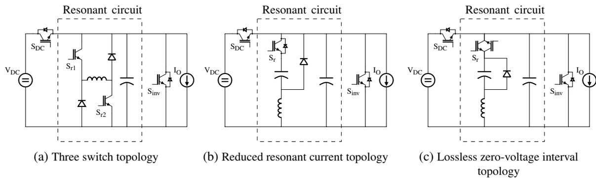
Fig. 3: Various circuit topologies of a Quasi-Resonant DC Link Inverter as described in [17]
