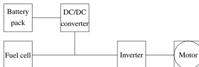
Fig. 1: A standard architecture example for multiple DC power source connection to the motor
