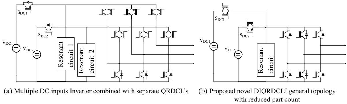
Fig. 4: Possible implementation of QRDCL in a dual input inverter
