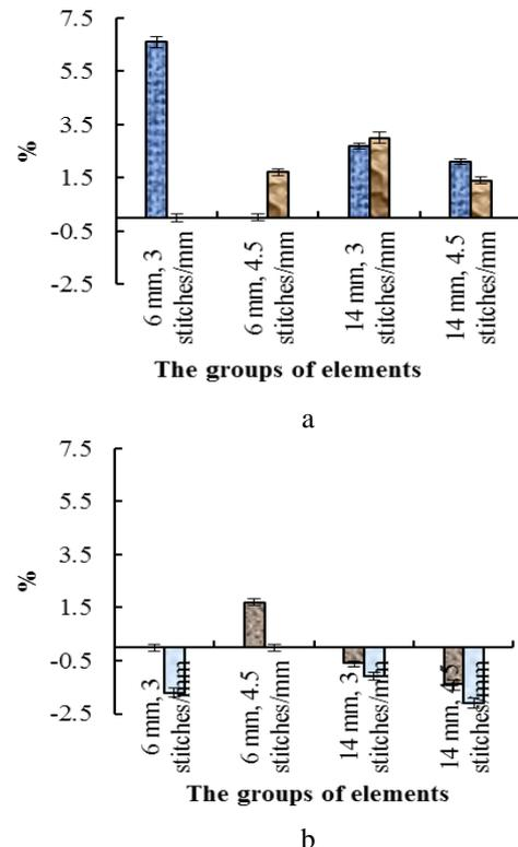
Fig. 2 The difference of the contour width CS of the electrically conductive embroidery elements in comparison to the designed size, when the contour width of the designed element is x axis, here: ■ – the section MN; ■ – the section OL; ■ – the section LM; ■ – the section ON; a – accomplished in warp direction; b – accomplished in weft direction
