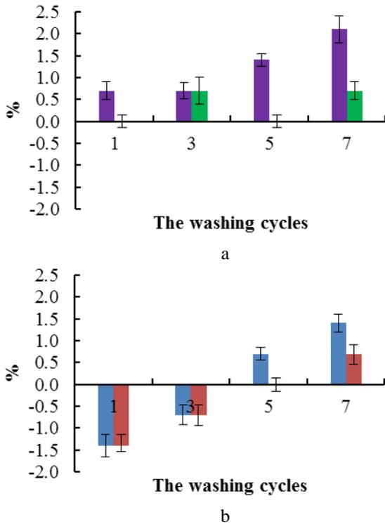
Fig. 5 The difference of the contour width CS of the electrically conductive embroidery element after the exploitation and the embroidered element when contour width is 14 mm and stitch density is 3 stitches/mm, when the width of the embroidery element is x axis, here:  $\blacksquare$  – the section MN;  $\blacksquare$  – the section OL;  $\blacksquare$  – the section LM;  $\blacksquare$  – the section ON; a – in warp direction; b – in weft direction
