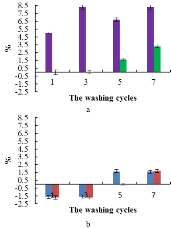
Fig. 4. The difference of the contour width CS of the electrically conductive embroidery element in comparison to the embroidered element when the contour width is 6 mm, when stitch density is 4.5 stitches/mm, when the width of the embroidery element is x axis, here: ■ – the section MN; ■ – the section OL; ■ – the section LM; ■ – the section ON; a – in warp direction; b – in weft direction
