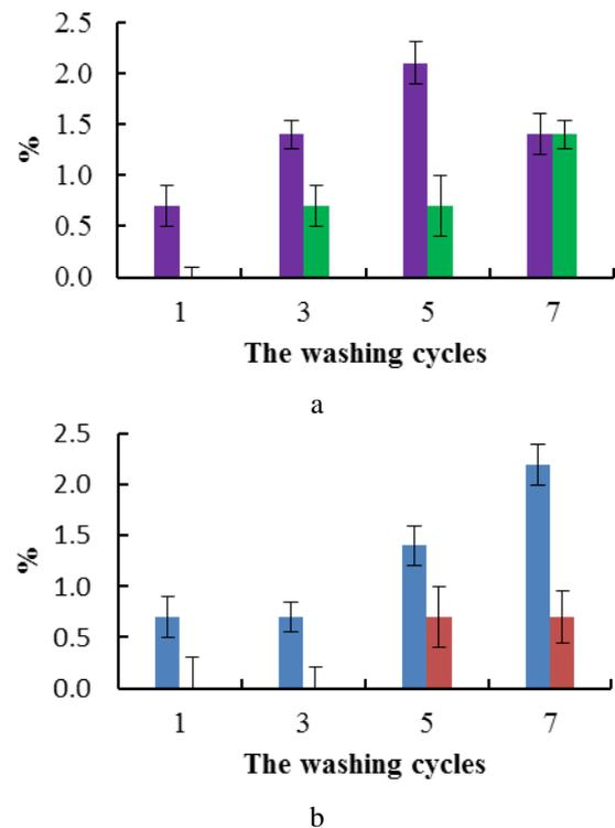
Fig. 6 The difference in the contour width CS of the electrically conductive closed-circuit embroidery element after the exploitation when contour width is 14 mm, when stitch density is 4.5 stitches/mm, here:  $\blacksquare$  – the section MN;  $\blacksquare$  – the section OL;  $\blacksquare$  – the section LM;  $\blacksquare$  – the section ON; a – in warp direction; b – in weft direction
