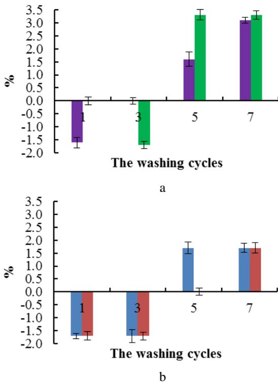
Fig. 3. The difference of the contour width CS of the electrically conductive embroidery element after the exploitation in comparison with the embroidered element when the contour width is 6 mm, when stitch density is 3 stitches/mm, when the contour width of the embroidered element is x axis, here: ■ – the section MN; ■ – the section OL; ■ – the section LM; ■ – the section ON; a – in warp direction; b – in weft direction
