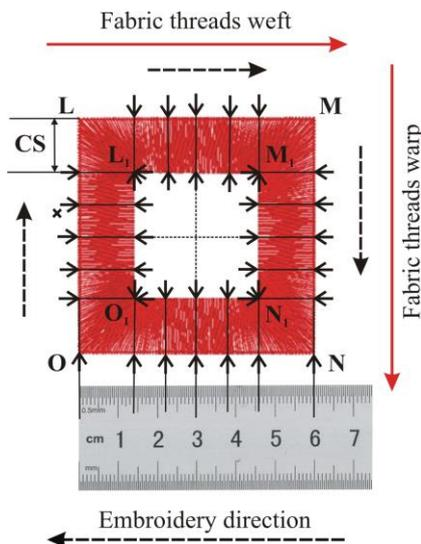
Fig. 1 The measurement scheme of the contour width of the electrically conductive element
