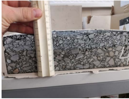
Fig. 7. Cut slab of sample for wheel tracking test
