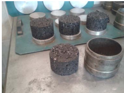
Fig.5. Marshall samples for optimising bitumen content
