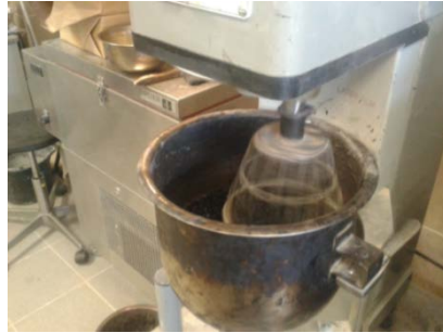
Fig.4. Asphalt concrete mixing equipment for optimising bitumen content
