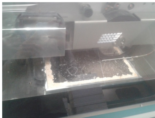
Fig. 6. Wheel tracking test equipment
