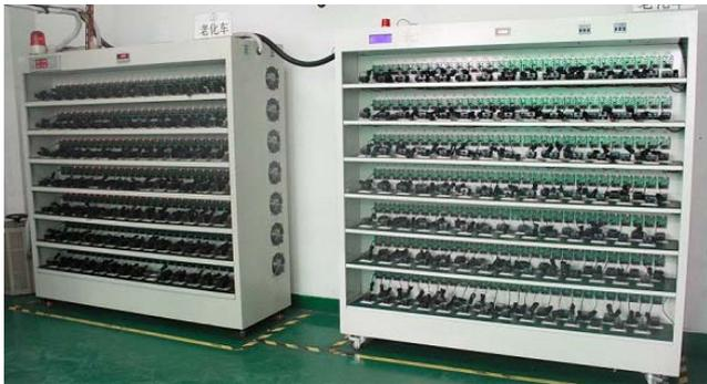
Fig. 4. Typical burn-in test setup in mass production of consumer-grade power supplies [43]
