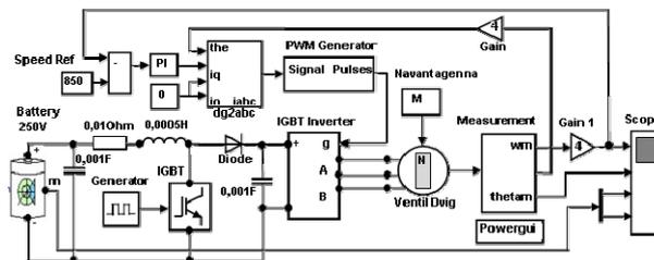
Fig. 2. Scheme of a simulation model of an electric drive system with a AC converter-fed motor
