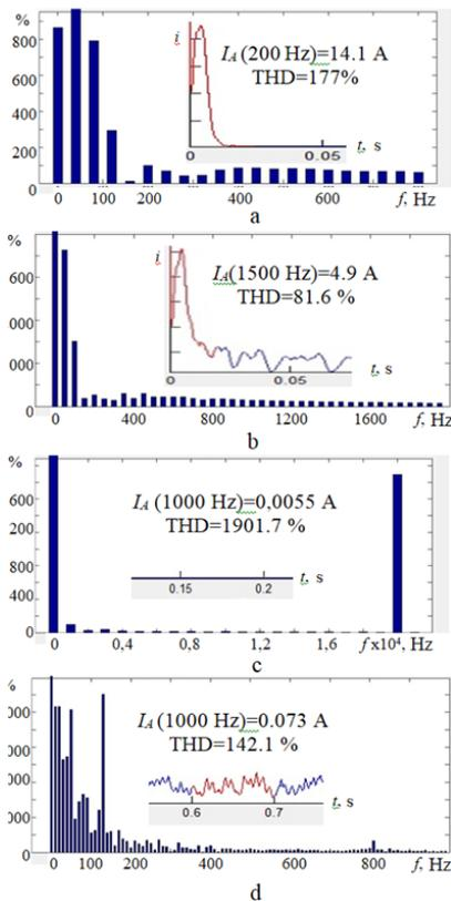
Fig.4. Spectral characteristics of the current functions in the HVB circuit in the AC converter-fed motor modes: a - start without load; b - start-up under load; c - idling; d - stationary load
