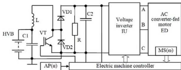
Fig. 1. Electric drive circuit with AC converter-fed motor
