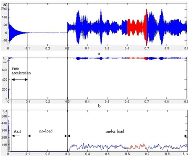
Fig.3. Functions of the output characteristics of the electric drive: a - torque on the motor shaft; b - rotor speed; c - current in the HVB circuit
