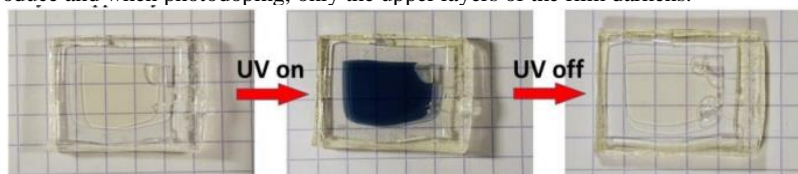
Figure 1. TiO 2 / PEGDA organogel sample exhibiting photodarkening and recovery.
